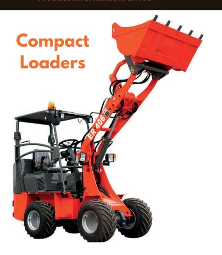
ER406 is a mini-wheel loader known for its compact design and maneuverability. This machine is perfectly suited for various types of projects, including use in small spaces as it has a width of 1.15m. The ER406 is equipped with a ROPS/FOPS-approved safety roof
