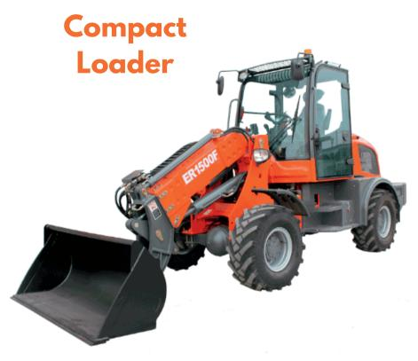
ER1500F is a telescopic wheel loader with 1500kg loading capacity. It is well-suited for work on a farm, in a warehouse or factory, on construction sites, and for tent installation and strike.
